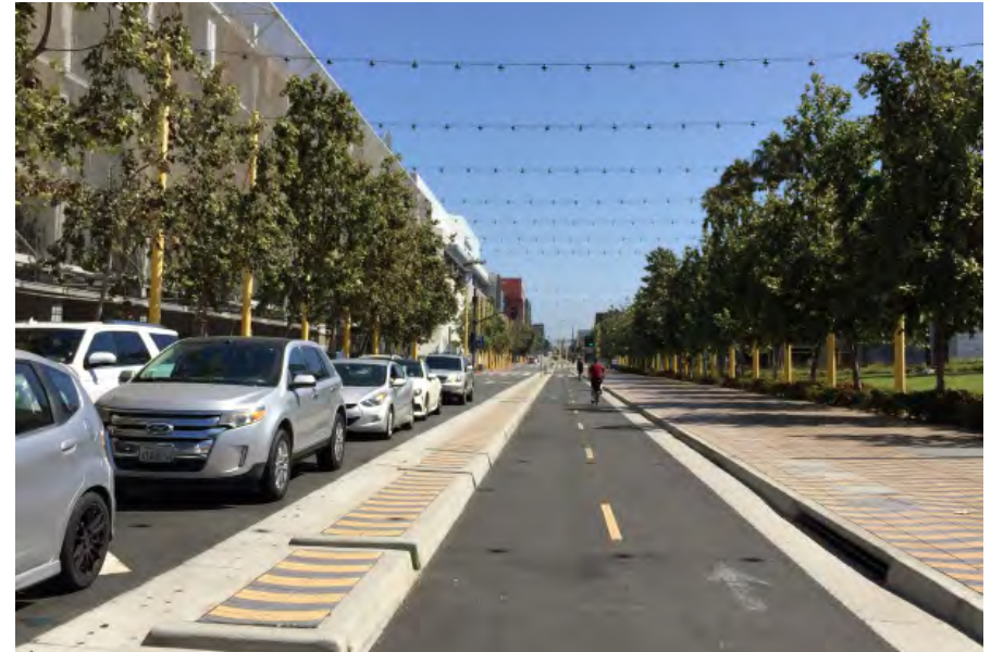
Figure 4.15: Two-Way Bike Path with Raised Buffer.
