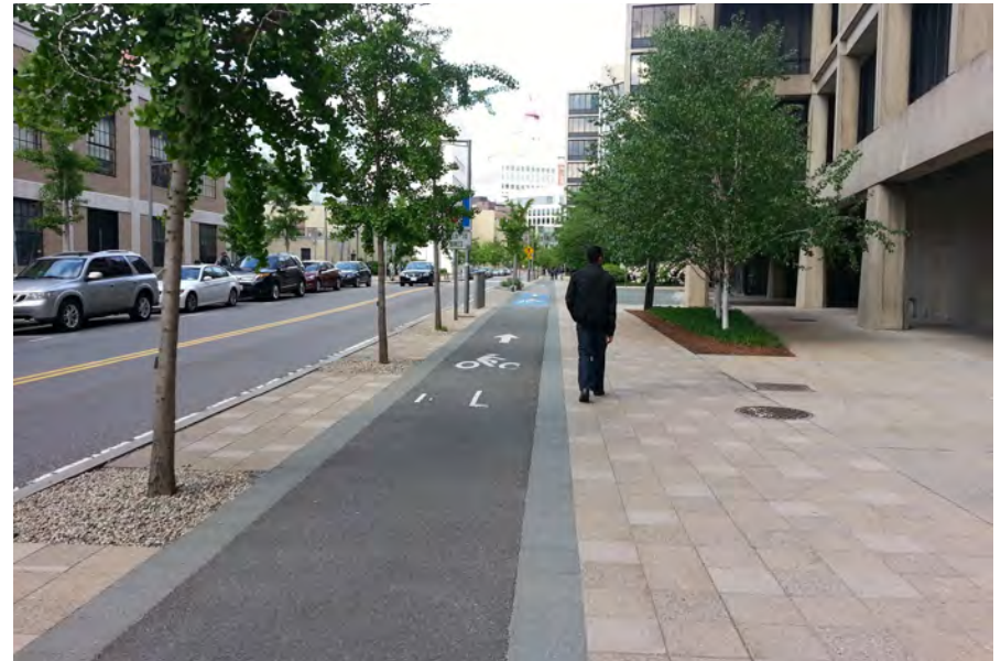
Figure 4.11: Multi-use Path with a Cycle Track Next to the Sidewalk.
