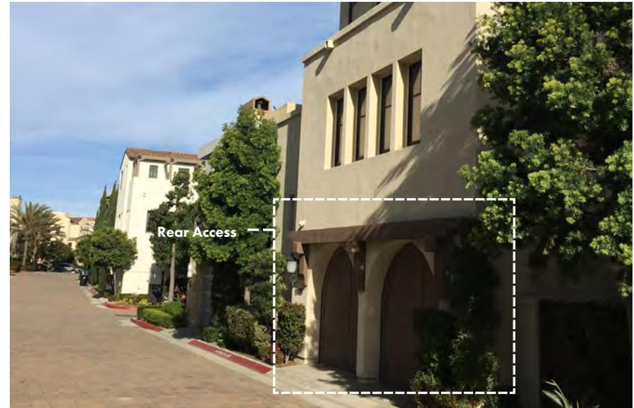
**Figure 3.10:** Example in a floodplain area of ground floor parking completely screened from view with decorative masonry ventilation blocks.
