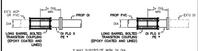
\* MAY SUBSTITUTE WITH 3X DIA C-900 and MJ X FLG ADAPTER
