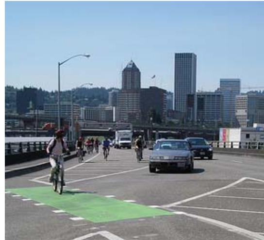
Figure 5-1: Colored Bicycle Lanes can increase driver awareness when they cross the path of bicyclists
